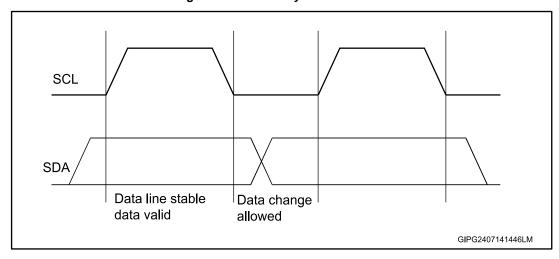
Figure 8: Timing diagram of I<sup>2</sup>C bus
