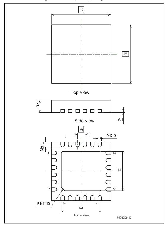
Table 16: QFN24L (4x4 mm) mechanical data
